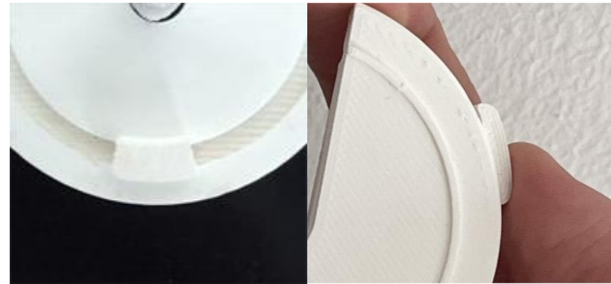
Figure 11 (left) , Top-side slider on token & Figure 12 (right) , First iteration slider on the side of the token
